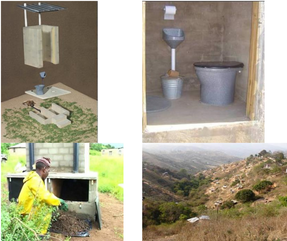
Figure 25: Model of dry urine diverting toilet in Durban, an interior of a UD toilet, emptying of a vault and the hilly terrains of eThekweni Municipality. Source: EWS.
